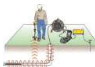
Find plastic pipe with integral line trace.
