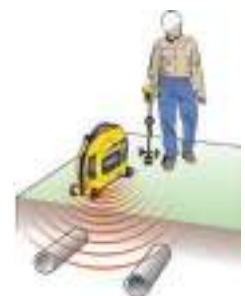
Induce a signal to locate utilities.
