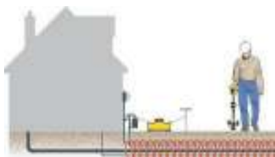
Direct connect to utility lines.
